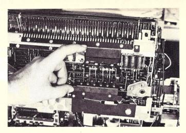
Photo 3. Exisiting screw holes are used to mount the solenoid assembly seen between my thumb and index finger.
